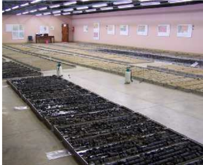
Figure 3: Well cores from the 1960s drilling for oil exploration are still being kept at the National Core Library at Donkerhoek outside Pretoria, managed by the Council for Geoscience
